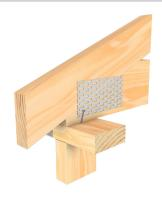
• Prevent the truss/rafter from moving along the top plate by Skew nailing the truss to the top plate.
