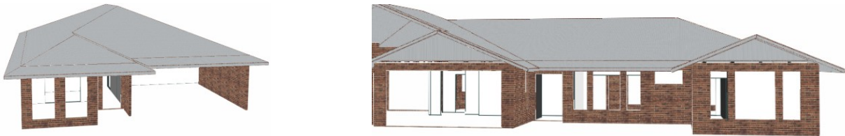
Fig 1 - Typical examples of front elevations with short walls where a PWTB would be best suited
