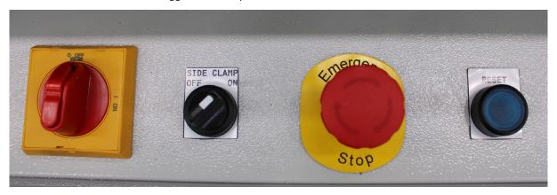
When the SCN machine is first turned ON, the reset push button illuminates to show that the emergency system requires resetting. Further, it also illuminates when the emergency system has been activated and then cleared. The RESET push button will require pressing to reset the machine.
