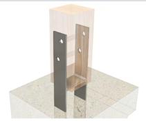
Drill through post using saddle holes to mark location.
