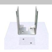
Drill two holes at marked location to required depth for selected hold-down bolt. Refer to bolt manufacturer guidelines for recommended pre-drill hole size and depth. Suggested minimum screw embedment depth 100mm or greater (Section detail shown above).
