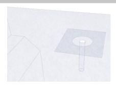
Drill single hole at marked location to required depth for selected hold-down bolt. Hole can be offset from center point within cut-out for adjustment purposes. Suggested minimum screw embedment depth 100mm or greater.
