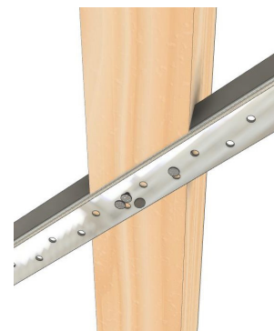
WRONG FIXING METHOD
