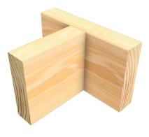
Position the supported beam to supporting beam, ensuring both beams are vertically plumb, and all edges are aligned.
