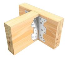
Position a pair of Multigrips at right angles on either side of the supported beam. Fix each Multigrip to each timber member with 5x3.15x35 Pryda Connector nails or 3 x No.12x35mm Pryda painted hex head screws.
