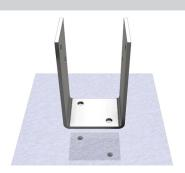
Drill two holes at marked location to required depth for selected hold-down bolt. Refer to bolt manufacturer guidelines for recommended pre-drill hole size and depth. Suggested minimum screw embedment depth 100mm or greater (Section detail shown above).
