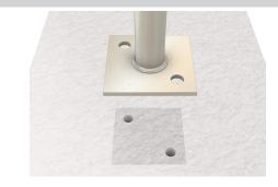
Drill two holes at marked location to required depth for selected hold-down bolt. Refer to bolt manufacturer guidelines for recommended pre-drill hole size and depth. Suggested minimum screw embedment depth 100mm or greater (Section detail shown above).
