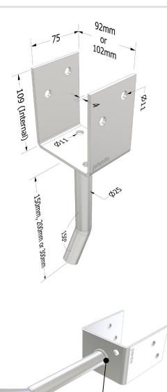
Fully welded solid stem to saddle.
