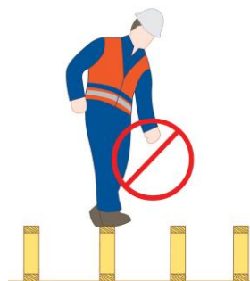
Figure 20: Don't walk on floor trusses until proper bracing is in place.
