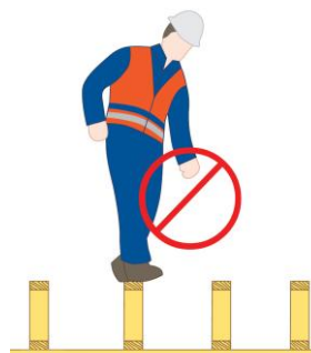
Figure 20: Don't walk on floor trusses until proper bracing is in place.
