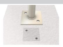
Drill two holes at marked location to required depth for selected hold-down bolt. Refer to bolt manufacturer guidelines for recommended pre-drill hole size and depth. Suggested minimum screw embedment depth 100mm or greater (Section detail shown above).
