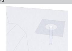
Drill single hole at marked location to required depth for selected hold-down bolt. Hole can be offset from center point within cut-out for adjustment purposes. Suggested minimum screw embedment depth 100mm or greater.
