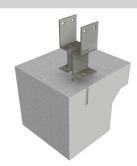
Drill two holes at marked location to required depth for selected hold-down bolt. Refer to bolt manufacturer guidelines for recommended pre-drill hole size and depth. Suggested minimum screw embedment depth 100mm (Section detail shown above).
